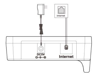
Note The base station should be used with original power adapter (5V/600mA) only. The use of the third-party power adapter may cause the damage to the base station.
