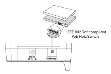
If in-line power is provided, you don't need to connect the AC adapter. Make sure the switch/hub is PoE compliant.
