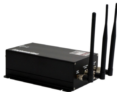
Two WIFI antennas and one mobile network antenna.
