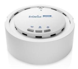
EAP350 is a 300Mbps wireless-n ceiling mount AP which offers users extended coverage, strong penetration, secure network management and simple connection.
