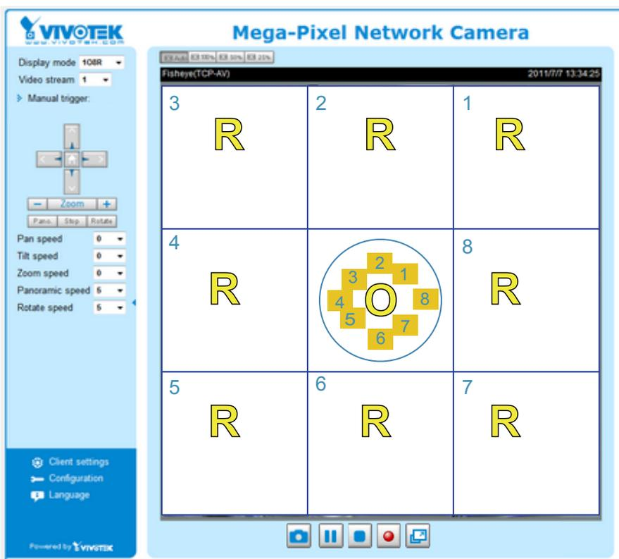
**Video Stream:** This Network Camera supports multiple streams (stream #1 ~ #3) simultaneously. You can select any one of them for live viewing. For more information about multiple streams, please refer to page 58 for detailed information.
