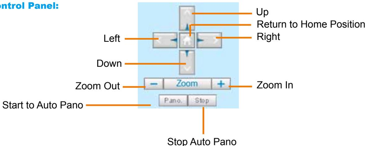
**Pano.:** Click this button to start the automated circular rotation through a regional view (360° continuous rotation). Note that this function does not apply in a Panoramic view because a Panoramic view already shows the full coverage.
