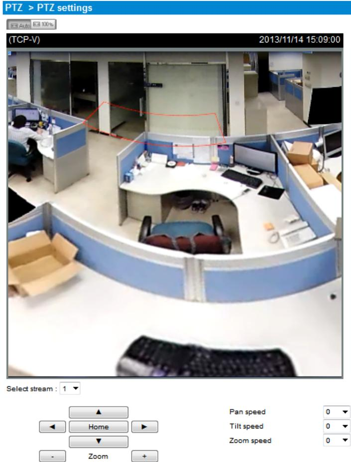
In this window, functional items related to the preset positions have been cancelled. This window is now used for changing the field of view when the Local dewarp function is applied to a video stream.
