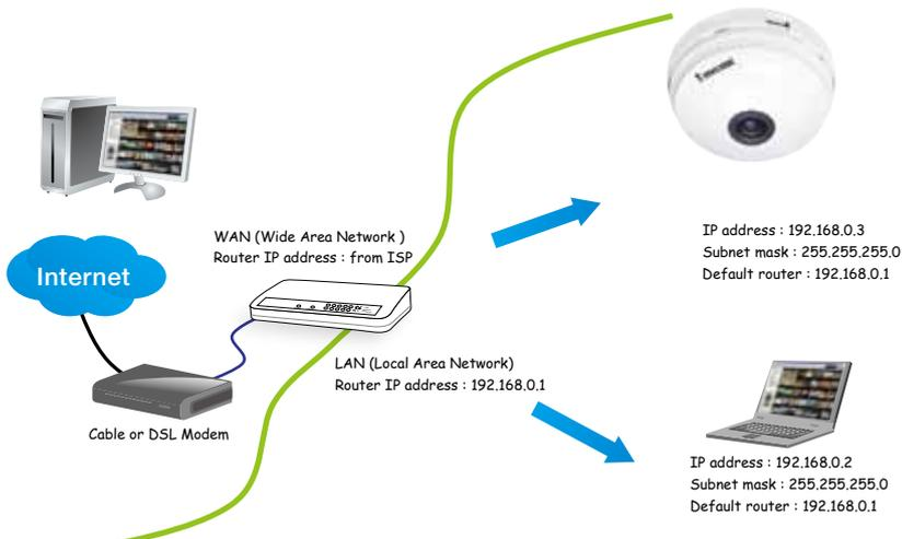
2. In this case, if the Local Area Network (LAN) IP address of your Network Camera is 192.168.0.3, please forward the following ports for the Network Camera on the router.
