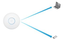
MU-MIMO with 3x3 and 1x1 clients: The UniFi AC HD AP communicates with one 3x3 client and one 1x1 client at a time.
