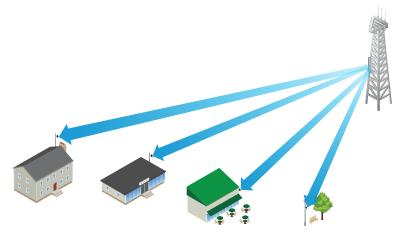
The PrismStation 5AC used as a CPE device for each client in an airMAX PtMP network.
