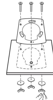
3 Secure the mounting bracket to the ceiling tile using three M3x30 pan-head screws, washers and wing nuts, as shown on the left.
