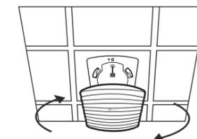
5 Connect the Ethernet cable to the ETHERNET port. Attach the EAP to the mounting bracket by aligning the arrow mark ▲ on the EAP with the arrow mark ▲ on the mounting bracket, then rotate the EAP until it locks into place, as shown on the left.
