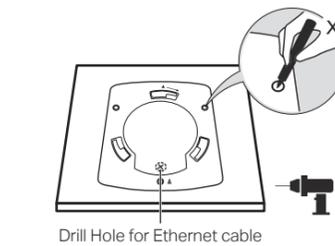
2 Place the mounting bracket in the center of the ceiling tile. Mark three positions for the screw holes and a position for the Ethernet cable hole. Drill three 4mm diameter holes for the screws and a 25mm diameter hole for the Ethernet cable at the marked positions.
