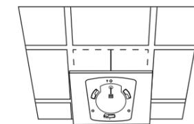
4 Feed the Ethernet cable through the hole and set the ceiling tile back into place.
