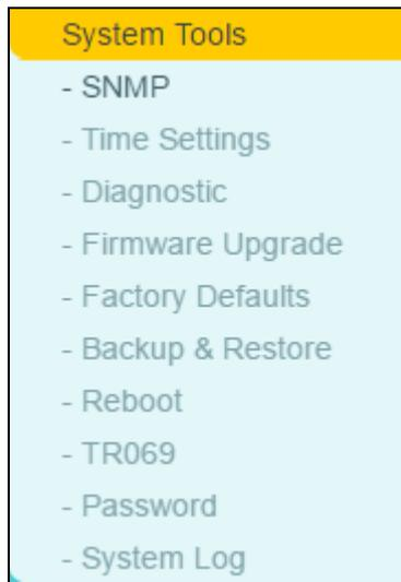
Choose [System Tools](#), and you can see the submenus under the main menu: [SNMP](#), [Time Settings](#), [Diagnostic](#), [Firmware Upgrade](#), [Factory Defaults](#), [Backup & Restore](#), [Reboot](#), [TR069](#), [Password](#) and [System Log](#). Click any of them, and you will be able to configure the corresponding function. The detailed explanations for each submenu are provided below.
