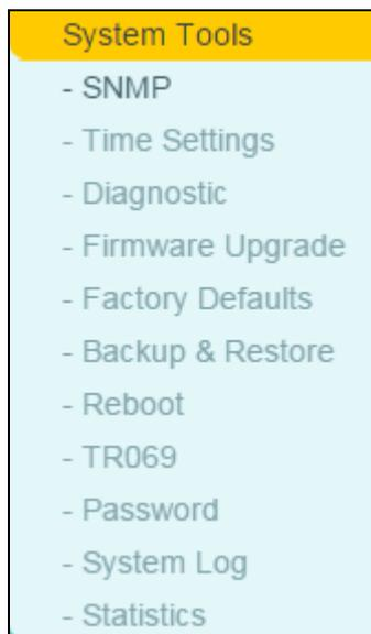
Choose menu [System Tools](#), and you can see the submenus under the main menu: [SNMP](#), [Time Settings](#), [Diagnostic](#), [Firmware Upgrade](#), [Factory Defaults](#), [Backup & Restore](#), [Reboot](#), [TR069](#), [Password](#), [System Log](#) and [Statistics](#). Click any of them, and you will be able to configure the corresponding function. The detailed explanations for each submenu are provided below.
