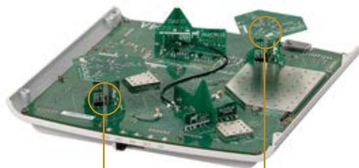
BeamFlex+ Adaptive Antenna Technology
