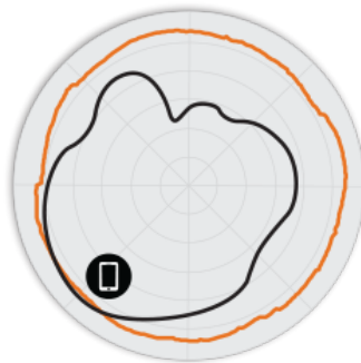
Figure 3. T710o 5GHz Azimuth Antenna Patterns
