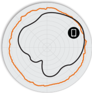
Figure 2. T710o 2.4GHz Azimuth Antenna Patterns
