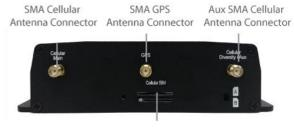
Redundant Cellular SIM Slot
