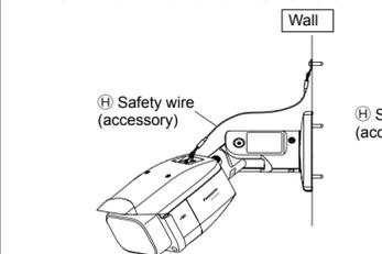
D) Using a 5 mm {3/16 inches} hex wrench (locally procured), loosen the Yawing lock screw, turn the camera until the sunshield faces up and adjust the tilt of the camera. (Yaw range: -115° to +200°)
