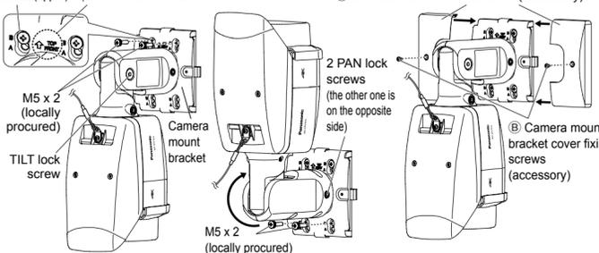
[1]-1 Loosen the TILT lock screw by about 1 turn until the camera faces downward and then temporarily tighten the TILT lock screw. After this, use the 2 upper M5 screws (locally procured) to secure the camera.
