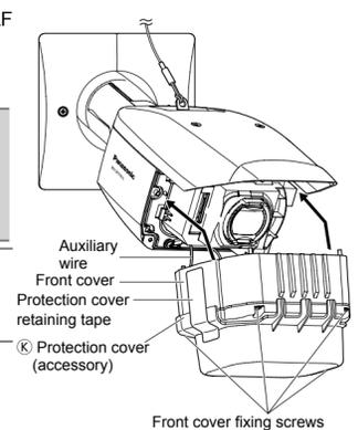
8 Secure the **H** safety wire (accessory) to the ceiling or wall.
