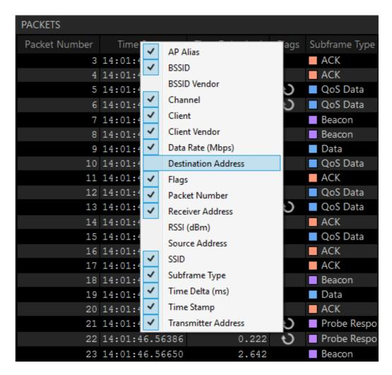
Eye P.A. will automatically remove columns as they become redundant due to the filtered data set. For example, if the BSSID is the same in every frame, it will no longer be represented in a column.
