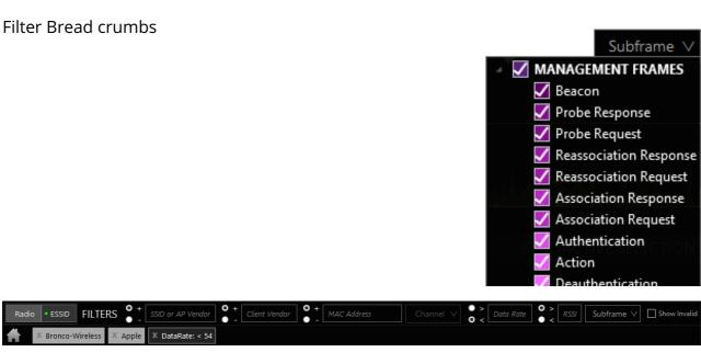
The filter bread crumbs represent the current requirements the user has manually entered as filters or navigated to by means of the multi-layered pie chart. To remove a crumb click the x. Bread crumbs will either be black to represent exclusive filters or gray to show inclusive filters.
