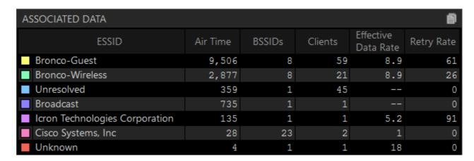
The Associated Data Table provides details for innermost ring of the multi-layered pie chart.
