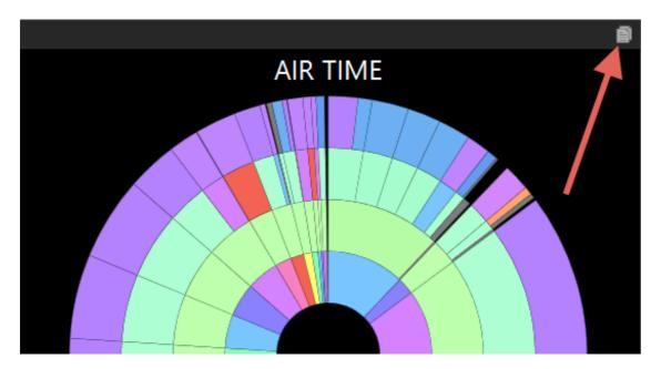
Eye P.A. contains a clipboard icon in each pane. Clicking this will copy the contents of the pane to the clipboard. The time graph and and treepies will be copied as images, while the active selection and associated data table will be copied as text, ready to paste into a text editor or spreadsheet application.
