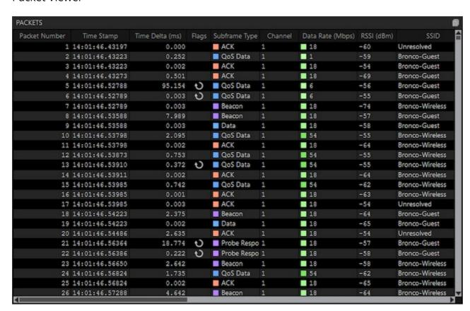
Eye P.A. will display the basic details of individual packets in the **Packets Table**, including **Subframe Type**, **RSSI**, **Data Rate**, and **Destination**. The user can define the columns in the packet viewer by right-clicking on a header and selecting the details they wish to view. Apply filters from the Filter Bar or use the treepie on the left to drill down into the packet viewer.
