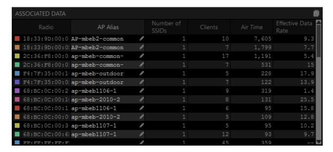
Each Line in the **Radio column** represents a group of SSID's on the same access point.
