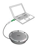
Plug the Jabra Speak 510 USB cable into any available USB port on your PC to charge the battery. The battery light is red when charging, and green for 1 minute when fully charged.
