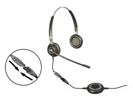
HOW TO CONNECT CONTROLLER TO HEADSET Plug the QD to the QD of any Jabra GN corded headset.
