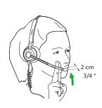
Jabra Engage 50 headsets have adjustable headbands for all-day comfort. The bendable 300° spin boom arm enables easy adjustment without risk of breakage. Place the microphone 2 cm away from the mouth for optimal positioning.
