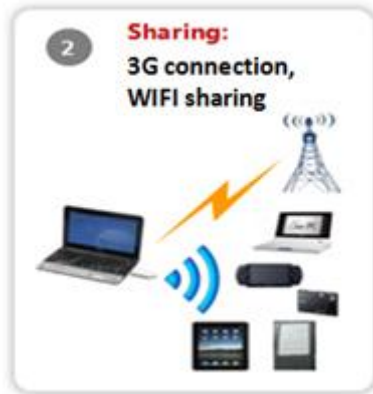
Figure 1-1 shows multi-devices access the wireless work through Wi-Fi and USB.
