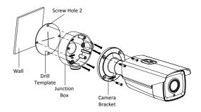
Figure 2-8 Installation with a Junction Box
