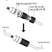
Figure 2-11 Water-proof Accessory Installation
