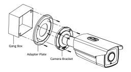
Figure 2-9 Installation with a Gang Box
