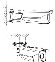
Figure 2-4 Install the Camera
