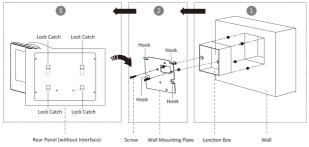
Figure 4-2 Wall Mounting with Junction Box
