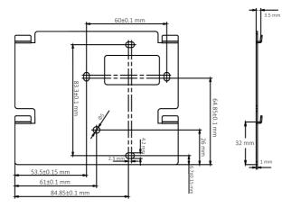
Figure 4-1 Wall Mounting Plate
