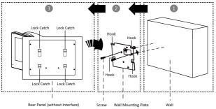
Figure 4-3 Wall Mounting without Junction Box
