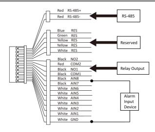
Figure 3-1 Wiring Description (Alarm Input Device)
