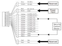
Figure 4-1 Wiring Description (Alarm Input Device)
