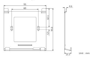
Figure 5-1 Wall Mounting Plate
