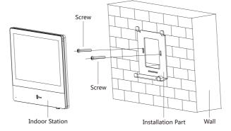
Figure 5-2 Installing the Plate
