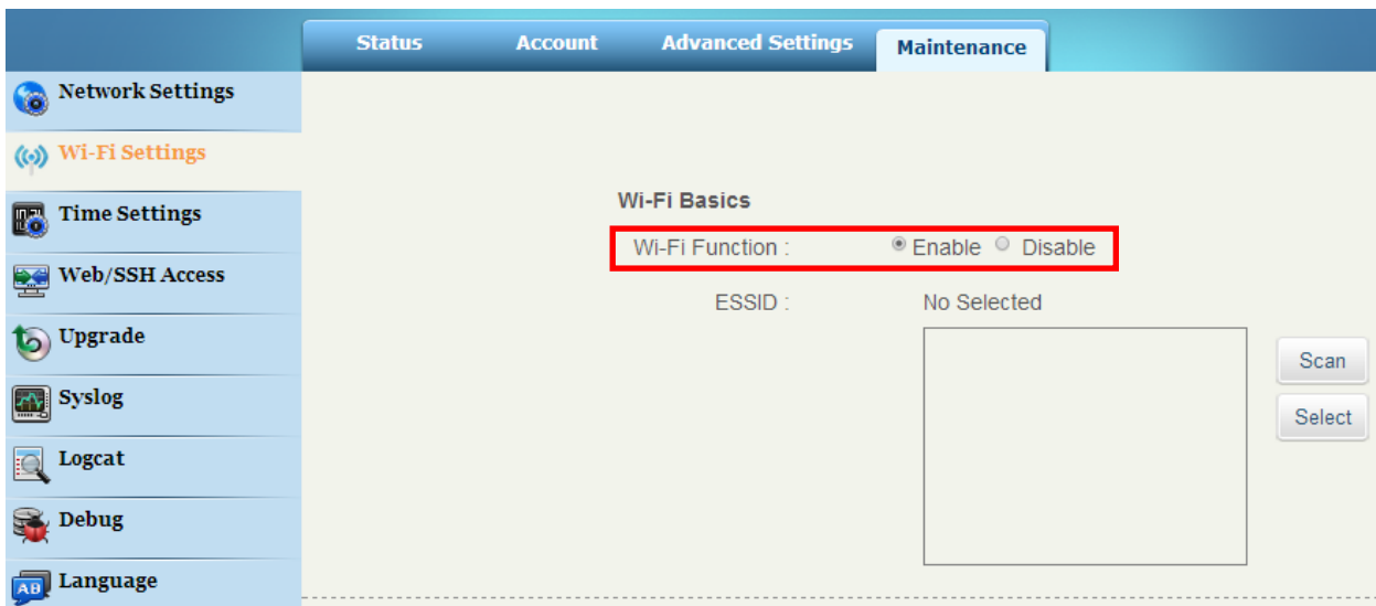
Figure 3: Turn On/Off Wi-Fi From Web UI
