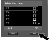
A list of all possible IP connections appears in the display (IP 1 to IP 6). VoIP connections that are already configured are marked with  $\[ egin{array}{c} \end{array} \]$ .
