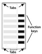
▶ Place the protective film back into the indented area so that the function keys fit into the recesses of the protective film. Then slide the protective film under the plastic tabs.
