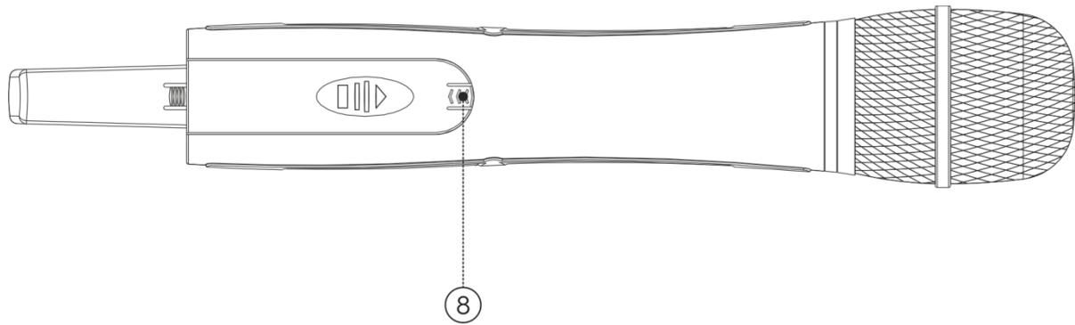
Two alkaline AA batteries are recommended. When inserting the batteries, observe the correct polarity as marked inside the battery compartment. When the LED is blinking (and the mic is not in pairing mode) please replace the batteries.
