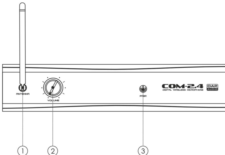
① Antenna: Position the antenna vertically
