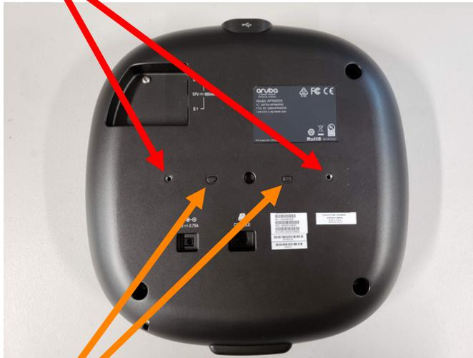
'Keyed' alignment knobs to ensure mount is properly installed.
