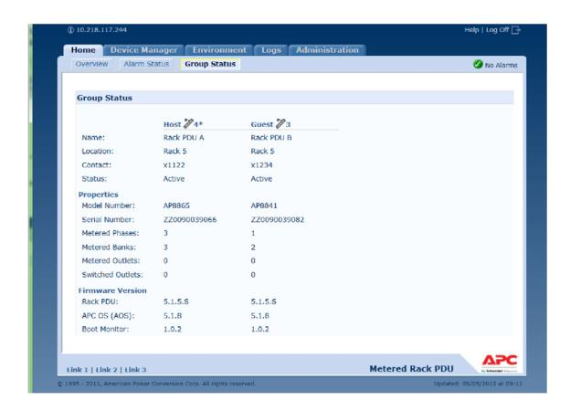
Most of the web pages under the Home, Device Manager, and Environment tabs allow you to switch between Rack PDUs for viewing status and configuration/control. This switching is accomplished by selecting the Rack PDU Display ID of the unit you would like to view. This is located at the top right of each table that supports multiple Rack PDUs. The Host Rack PDU that you are logged into is always denoted with an asterisk (\*) following the Display ID.
