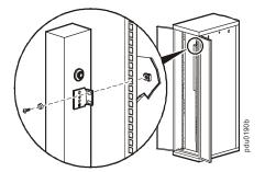
**Horizontal mounting.** You can mount the Rack PDU in a 19-inch NetShelter or other EIA-310-D standard 19-inch rack:
