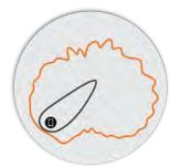
Note: The outer trace represents the composite RF footprint of all possible BeamFlex antenna patterns, while the inner trace represents one BeamFlex antenna pattern within the composite outer trace.
