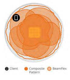
Figure 2. R350 2.4GHz Azimuth Antenna Patterns
