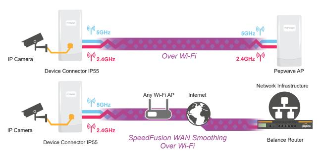
Using the Device Connector IP55, the IP camera is able to upload videos using both the 5GHz and 2.4GHz frequencies at the same time. If one frequency loses connectivity, the other will seamlessly take over. If the network is using an AP from another vendor,
